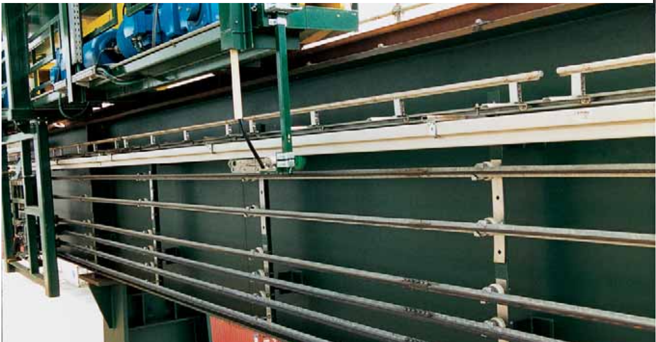
Antenna support arm assembly for a large crane application.
